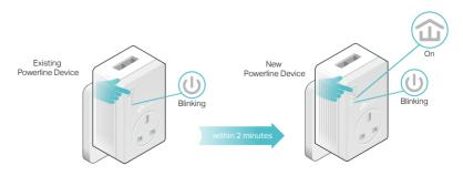
**3.** Relocate the new powerline adapter to the place where wired internet access is needed.
